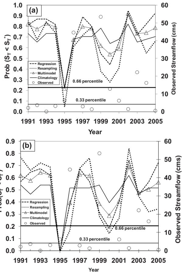
**Fig. 5.** Role of streamflow forecasts in predicting the end of the season target storage that corresponds to the stage of 72.1 m, mean sea level. (a) Normal water quality release of 7.8 cms. (b) Restricted water quality release of 2.8 cms. Note that the multimodel forecasts clearly suggest increased risk of not meeting the target storage in comparison to the risks suggested by the climatology during below-normal years.
