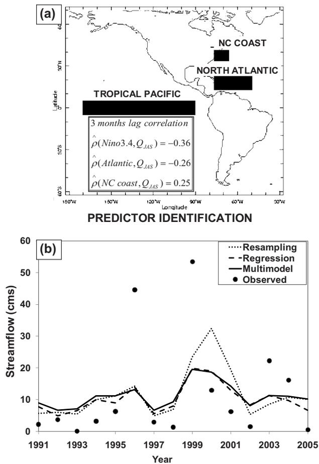
**Fig. 3.** Leave one out cross-validated seasonal (JAS) streamflow forecasts for the Falls Lake from three forecasting models [(b) regression, resampling, and multimodel] along with the employed predictors (a). Principal components of the three SST regions [shown as rectangles in (a)] were performed and the dominant two components were employed for developing the streamflow forecasts represented in the form of ensembles.
