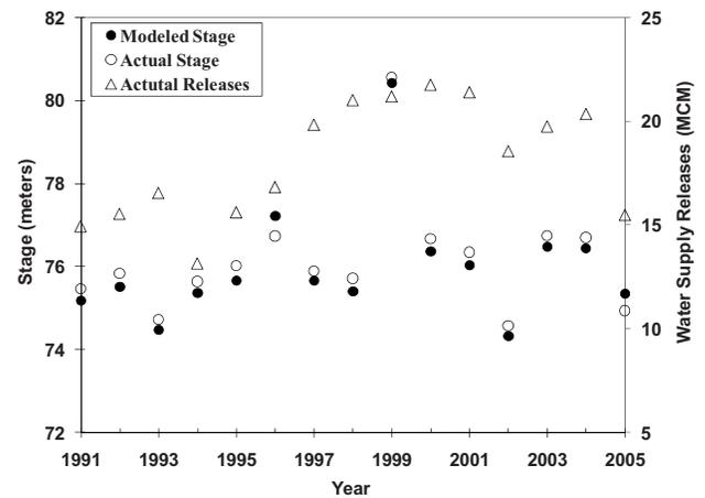
**Fig. 2.** Comparison of modeled stages with the observed stages in September for the period 1991–2005. The reported water supply releases during JAS from Falls Lake are also shown. Modeled stages are obtained upon simulating the model with observed flows, releases, and by forcing the model with the initial storage recorded each year on July 1.
