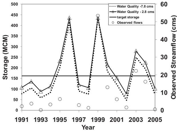
**Fig. 4.** Modeled storages for two water quality release scenarios: normal (7.8 cms) and drought (2.8 cms) conditions along with the observed streamflows and the target storage (solid horizontal line). The storages shown are obtained by combining the observed streamflows with the chosen water quality release and the corresponding year's summer water supply release in Fig. 2.
