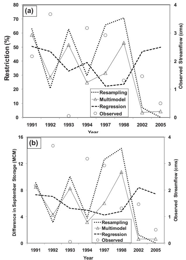
**Fig. 7.** Performance of streamflow forecasts in suggesting restriction for the prescribed level of reduction in the risk (5%) of not attaining end of the season target storage (a) and in improving the end of the season target stage (b) (upon validating with observed flows) for the obtained restriction in (a)
